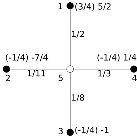
Figure 1: Electrical network of a  $\star_4$  graph with vertex labels to the left of/below the vertices (boundary vertices are solid black while the interior vertex is white), current in parentheses, electric potential to the right of current, and conductivities to the left of/below the edges connecting the vertices.
